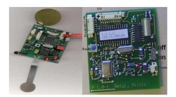
Figure 1: The two modules that combined make up the Smart-It unit: Left, the sensor module with light sensor, microphone, 2 accelerometers, thermometer, pressure sensor (bottom) and buzzer (top). Right, the wireless communication module. Both boards measure  $43 \times 50$  mm.
